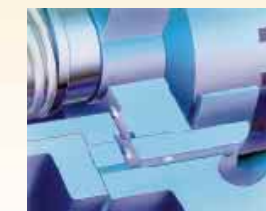
Oversize Seal Chamber with Seal Vent System Large seal cavity design allows easy conversion to a wide variety of single and multiple seal types and configurations. Internal seal vent system reduces seal face load and provides continuous cooling for extended service life.
