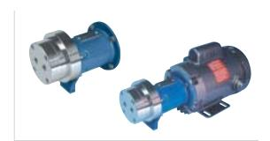
Liquiflo's 4-Series pumps are low-flow/highpressure magnetically-driven gear pumps that are completely field repairable. The 4-Series housings are manufactured from Bar Stock in 316 Stainless Steel, Alloy-C or Titanium. With several material options for shafts, gears, wear plates and bearings, these pumps can be used in a wide variety of chemical processing applications.
